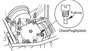
Figure 7-11 Transmission Drive Gearbox
